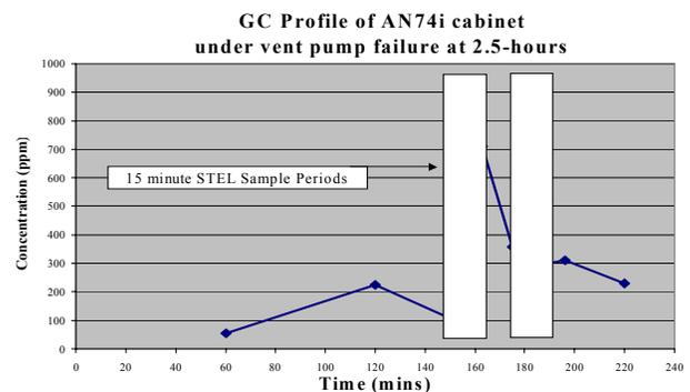
A gas chromatograph (GC) was used to test the concentration of ethylene oxide in the air samples.
